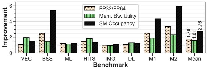
Fig. 10: Hardware metric improvement gained by *KeSCo* in different benchmarks, under the setting where *KeSCo* achieves the highest speedup.
